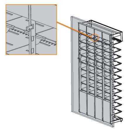
Alternative mounting method: using wire cable, wall mount, screws and anchors.
