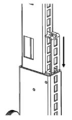
Slot Extension Bracket allows for a shelf to be placed at the point where the Infinity Fixture telescopes.
